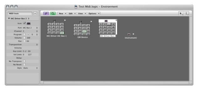
Here, two new Multi Instruments have been created from the "New" menu. When each is clicked on its settings are shown in the Inspector panel at the left hand side.
