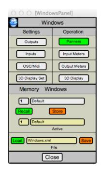
The most useful windows can be opened and closed by clicking on the named buttons. Any opened windows can then be dragged around the screen to desired positions. The result can be stored to one of ten memory locations. The white number box above "Recall" is used to set the number of the memory location. "Store" will then store it, with an option to name, or rename, the memory location.
