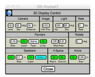
The user can change the vertical position, lens angle and distance of the "Camera". You can also move the vertical position of the whole image and rotate it, change the position of the lighting, and the "Frame Rate".
