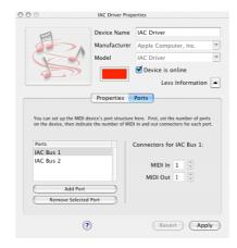
Here the first port has been re-named "IAC Bus 1" by double clicking on the name and re-typing. A second port has been added by clicking on "Add Port", and it has been been re-named as "IAC Bus 2". Each port can handle 16 Midi channels.
