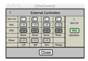
For the sake of simplicity Panner 1 is controlled by controllers on Midi channel 1, Panner 2 by controllers on Midi channel 2 etc. up to Midi channel 16. Each channel will need to have its Midi controller information set up separately.
