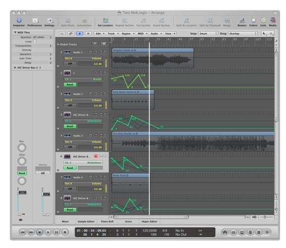
The picture above shows four mono audio tracks and four Midi tracks that control the movements of the associated panners in 3DAudioScape.
