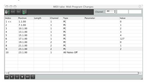
Items can be added to the list with the "Add" button, and deleted with the "Del" button. The position of the event can be edited by double clicking in the "Position" box, and typing. Similarly, the Midi channel, message type and value can be edited.
