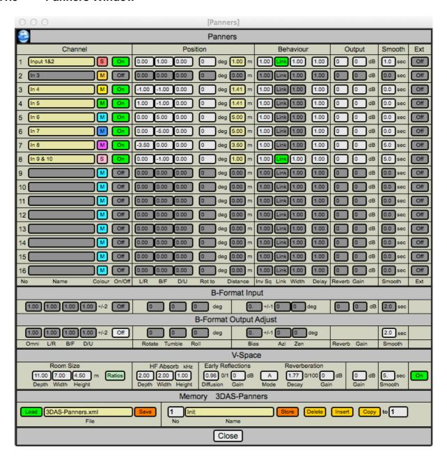
This window controls the sixteen "panners" for mono and stereo signals and the "V-Space" reverberation engine. In the ambisonic version it also controls the four-channel B-Format input and the total B-Format sound field.
