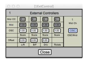
The "OSC/Midi" switch in the right-hand panel selects whether the panner is to be controlled by OSC or Midi Controller. The settings for the one not chosen are greyed out.
