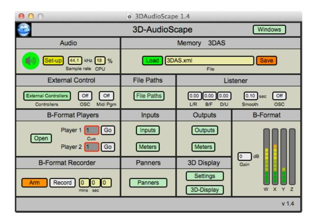
Light green buttons open windows for detailed operations and settings for the function named on the button.
