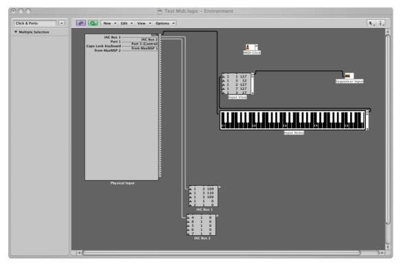
Curiously, by default Logic routes the outputs of the "IAC Driver Bus 1" and "IAC Driver Bus 2" Multi Instruments to the "Physical Input" and back into the "Sequencer Input", creating a Midi loop, which causes all
