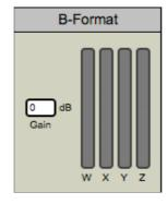
The meters show the levels of the W, X, Y and Z components of the internal B-Format signal, which is wired to the "B-Format Recorder", and to the "Decoder", which is set up in the "Outputs" window. The "Gain" box controls the output level.
