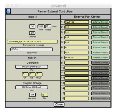
The left-hand side of this page sets the general properties of OSC and Midi messages, while the right-hand side has buttons which opens a more detailed set up window for each panner.
