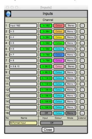
The "Input" box is a menu where the input to the each panner can be selected. These are selected as stereo inputs. Options are: Off, In 1&2 to In 15&16. These are the analogue or digital inputs of the attached audio interface.
