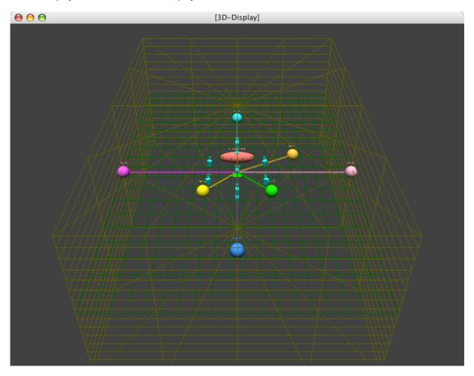
This contains a composite display of each sound source, each loudspeaker, and the virtual room set up in the "V-Space panel" (See Sec. 4.1.3).
